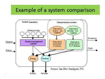
In this example different treatment systems are compared regarding their consumption of material and energy and the emissions and costs associated to the system.
